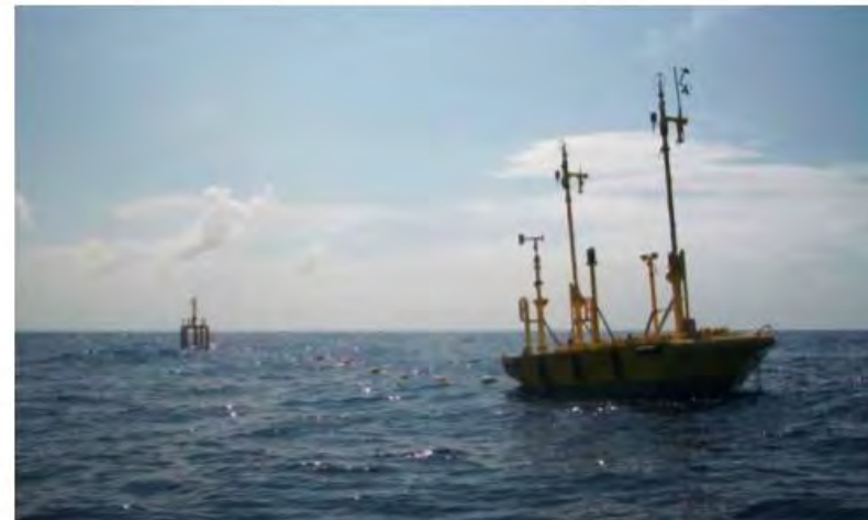
EASI-ASIS Buoy in tandem mooring
